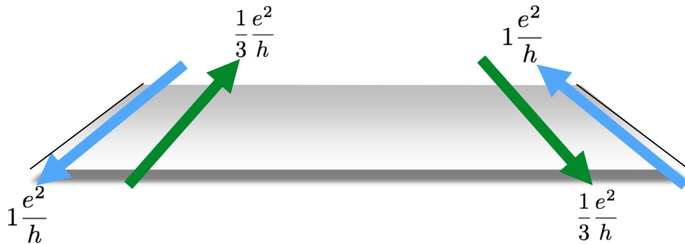
naive model 2-probe conductance =  $4/3 e^2/h$
