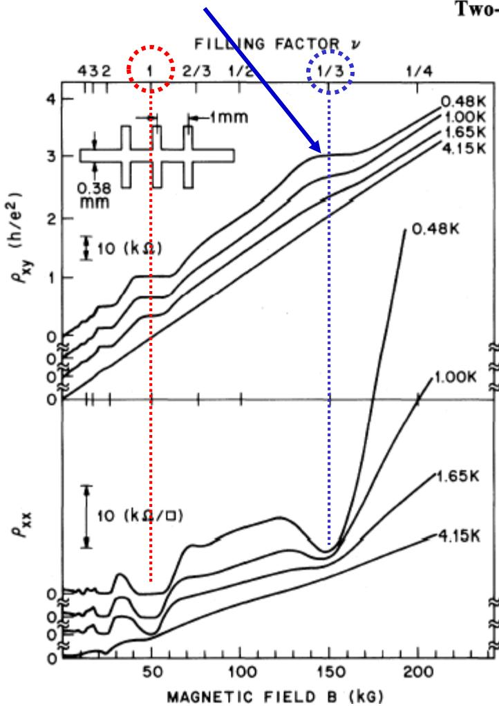
tion. Our observation of a quantized Hall resistance of  $3h/e^2$  at  $\nu = \frac{1}{3}$  is a case where Laughlin's argument breaks down. If we attribute it to the presence of a gap at  $E_F$  when  $\frac{1}{3}$  of the lowest Landau level is occupied, his argument will lead to quasiparticles with fractional electronic charge of  $\frac{1}{3}$ , as has been suggested for  $\frac{1}{3}$ -filled quasi one-dimensional systems.<sup>21</sup>
