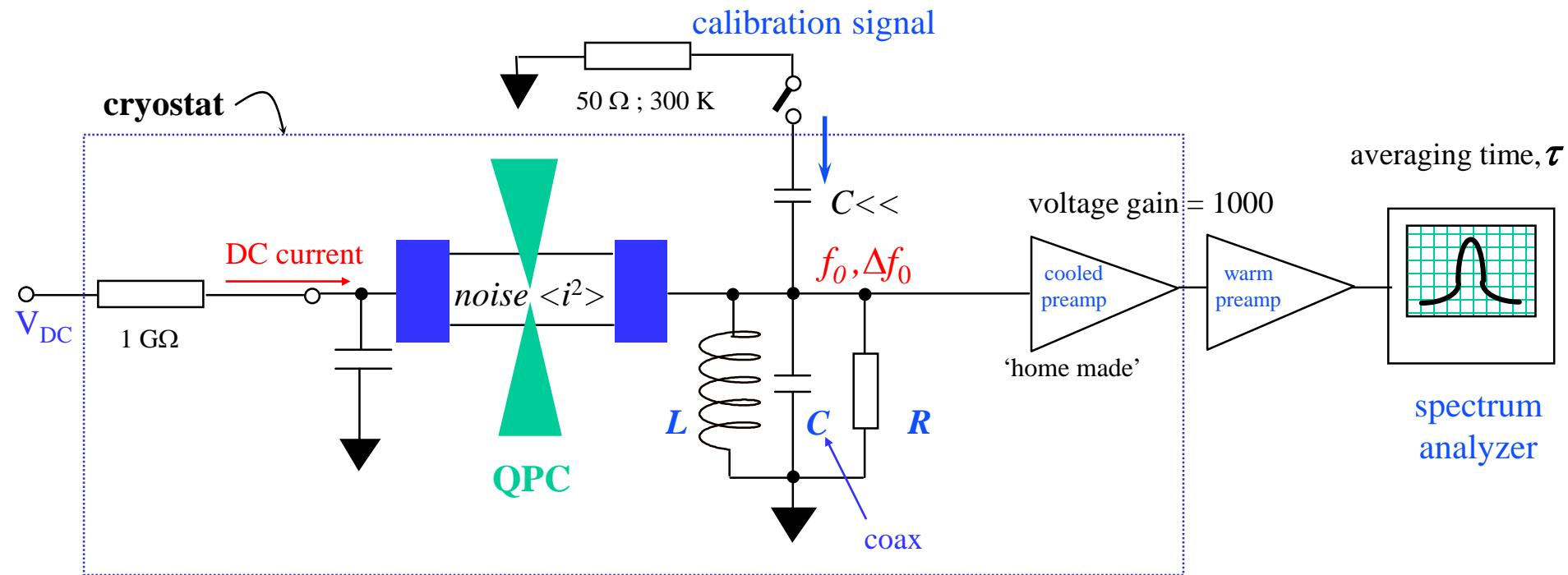
$$f_0 = \frac{1}{2\pi\sqrt{LC}} \approx 2 \rightarrow 4\text{ MHz} \quad , \quad \Delta f_0 = \frac{1}{2\pi RC} \approx 30\text{ kHz}$$
