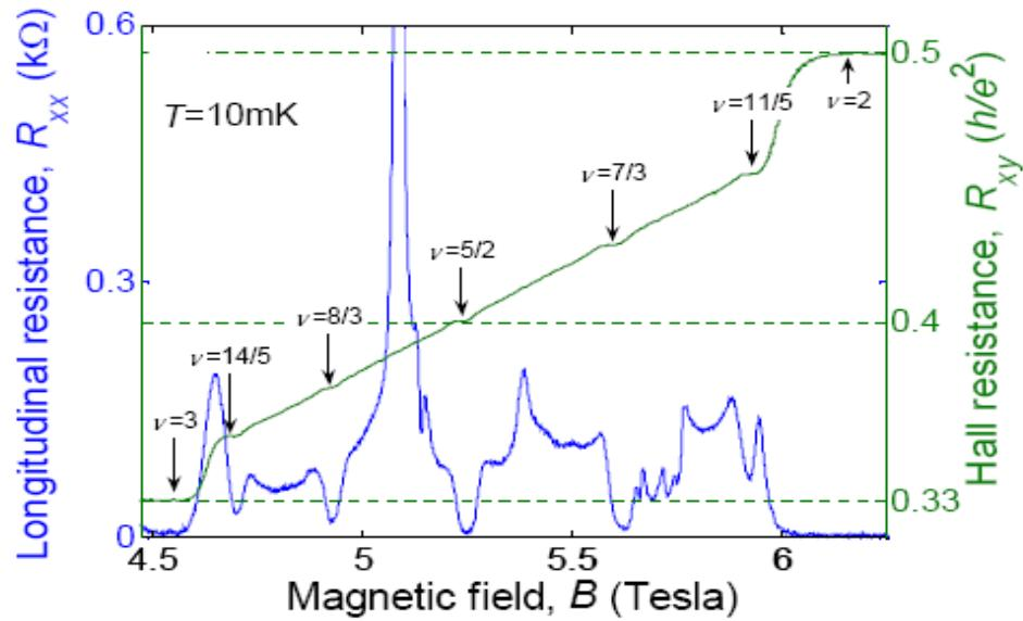
$$n_e = 3.2 \times 10^{11} \text{ cm}^{-2} \quad \mu = 30.5 \times 10^6 \text{ cm}^2/\text{V-sec}$$
