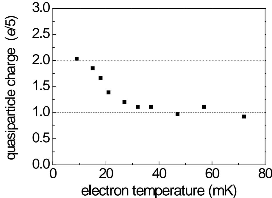
*bunching* of quasiparticles at low temperatures
